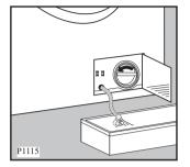
• Remove any objects from the pump impeller by rotating it.
